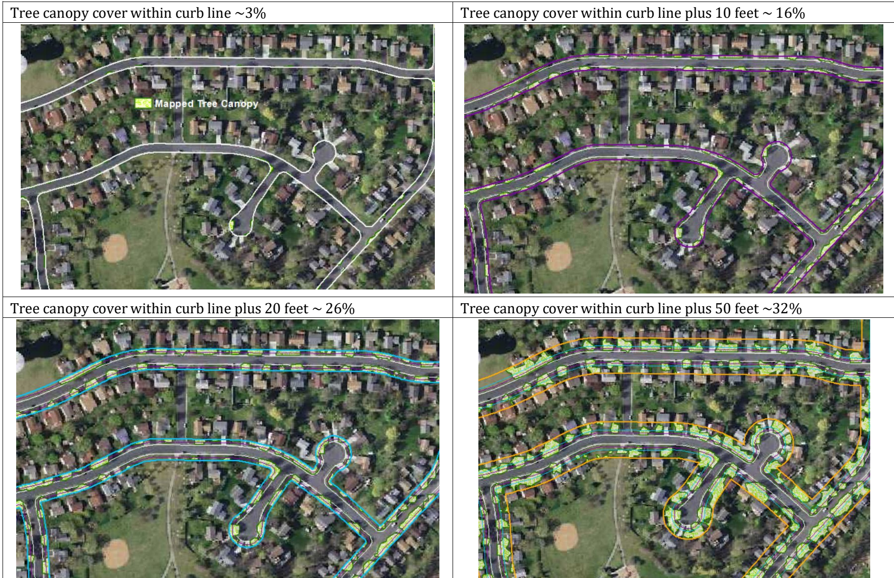
Figure 2. Percent tree canopy cover quantified over and within variable distances from the curb line.
