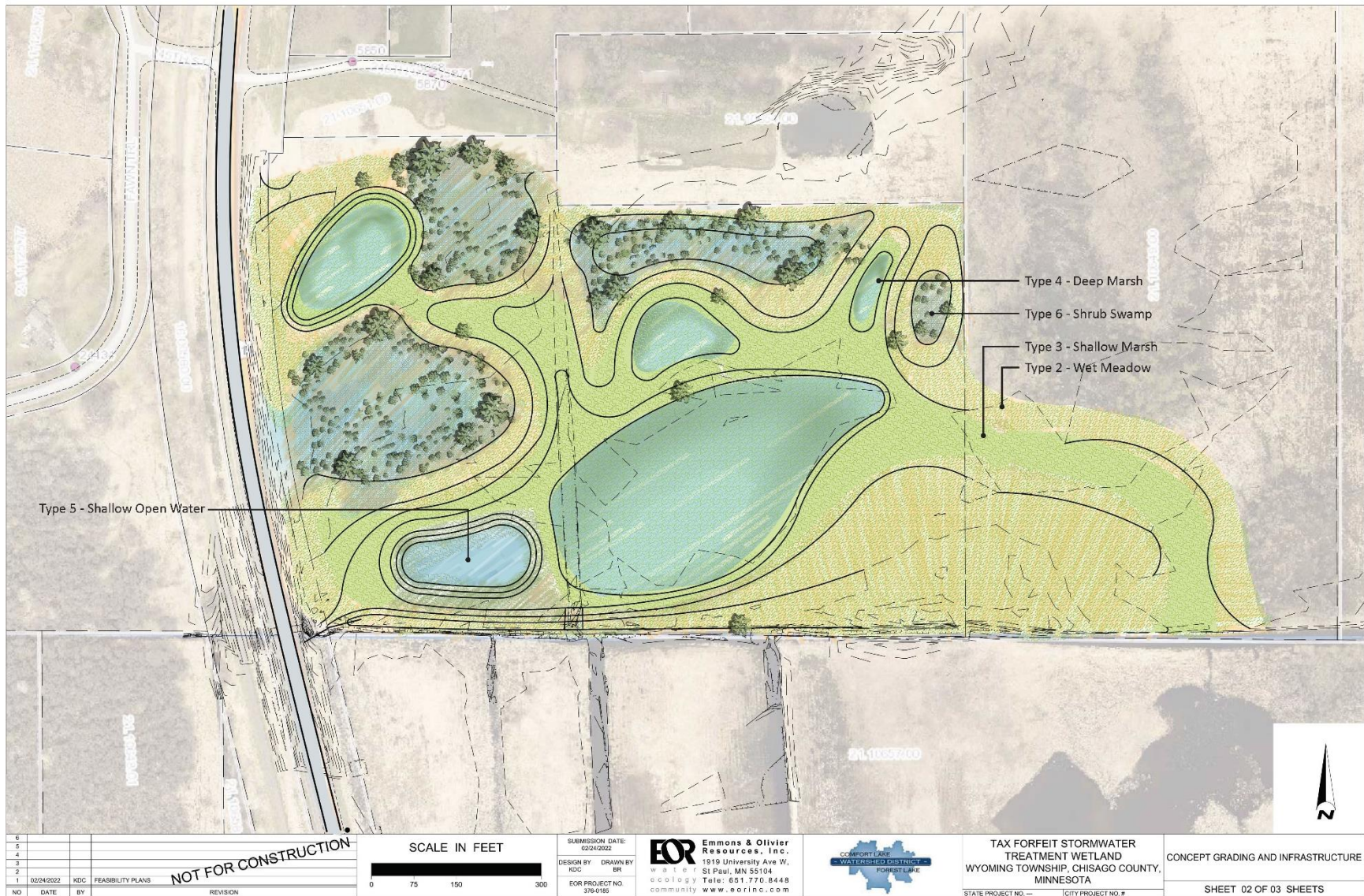
Figure 3. Rendering of concept plan illustrating proposed wetland types and habitat.
